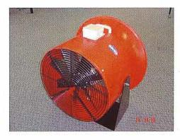
The Portable Axial Fan is specifically designed to provide air movement and ventilation in a variety of situations. The fan casing is moulded from plastic. The motor and bracket are aluminium and the adjustable pitch impeller is polypropylene. The high efficiency impeller with eight wings provides for a very high air flow of 6300 m<sup>3</sup>/hr.
